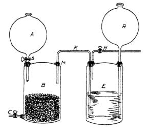
bubbling up through the water in E. At the same time the pressure of the gas collecting in E will force the water up into R. By turning the stop-cock H, a supply of gas is received under the pressure of the head of water in R. If an excess of acid is permitted to flow out of the separatory funnel the gas generated by it will be stored in E ready for the next time it is to be used.
